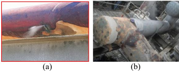
Fig. 3. Two damages in the fractionator overhead vapor line shown in Fig. 2.
