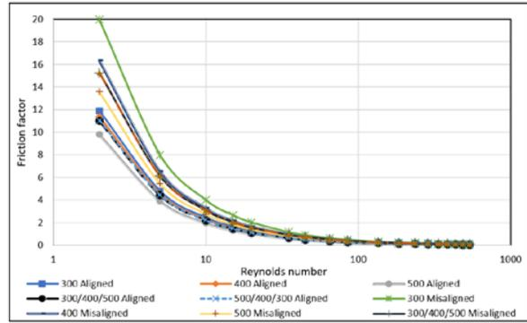
Fig. 7. Comparison of friction factor vs Reynolds number for aligned and misaligned mesh configuration for uniform mesh.
