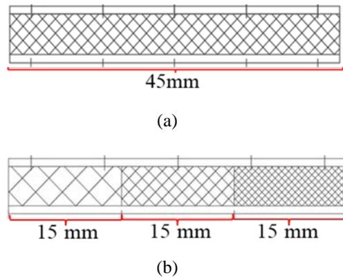
Fig. 2. Types of Stirling regenerator matrix. (a) Uniform wire mesh regenerator (b) Hybrid wire mesh regenerator
