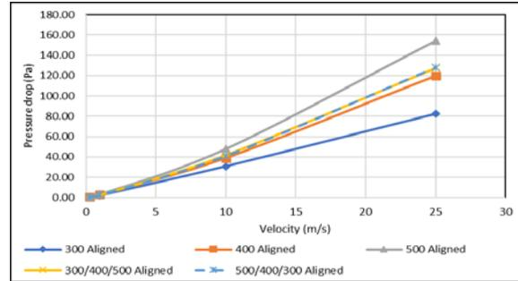
Fig 5. Pressure drops vs velocity for aligned configuration for uniform mesh regenerator.
