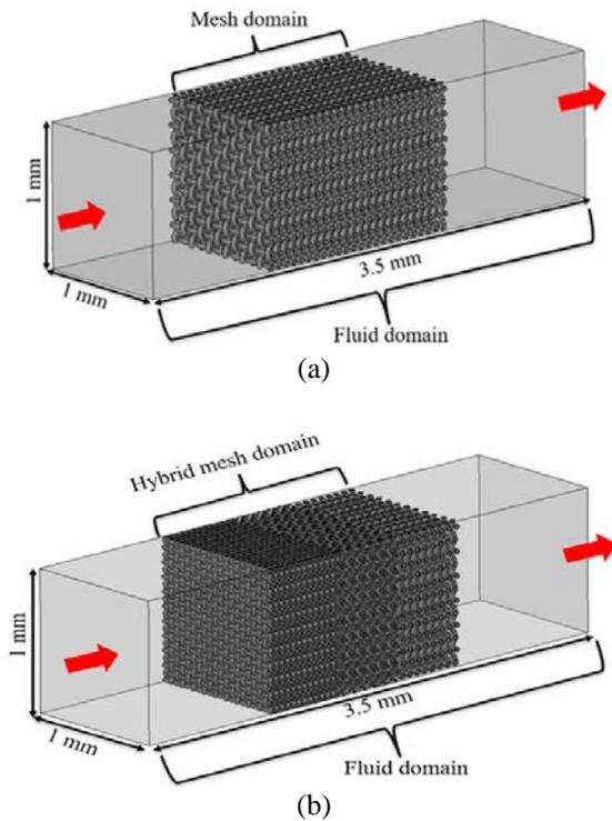
Fig. 3. 3-D view of the grid layout for the computational domain; (a) Uniform mesh and (b) Hybrid mesh configuration.
