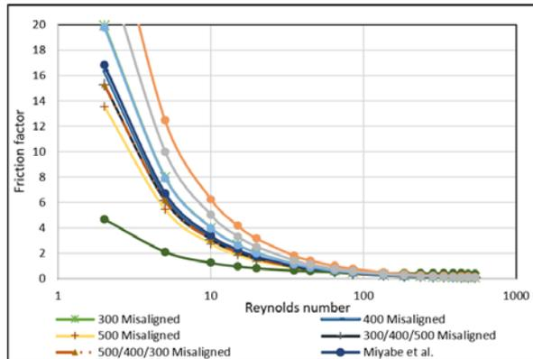
Fig. 8. Comparison of CFD friction factor with another researcher.
