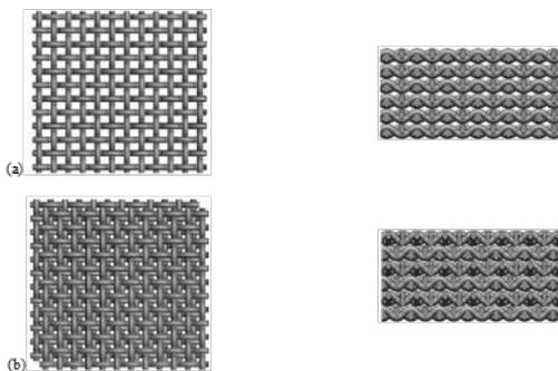
Fig. 1. Design layouts of stacked wire mesh screens (a) stacked aligned and (b) stacked misaligned configurations.
