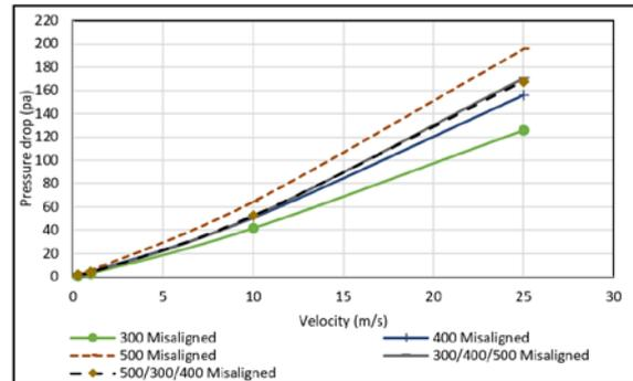
Fig. 6. Pressure drops vs velocity for misaligned mesh configuration for uniform mesh regenerator.
