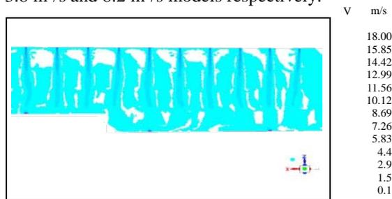
Fig. 9. Air velocity magnitude contours at y1.6m in 3.8 m<sup>3</sup>/s air distribution model
