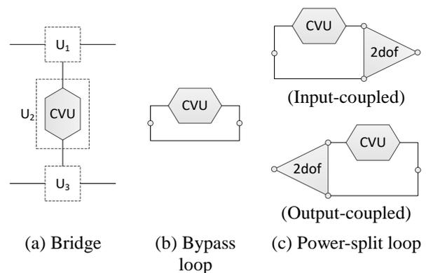
Fig. 1. Required structures for dual-way manipulated systems, bypass-type dual-path systems, and power-split-type dual-path systems in a BPG
