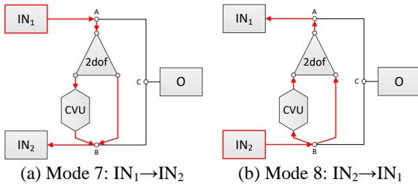
Fig. 10. Power flow patterns for neutral modes with internal power flow
