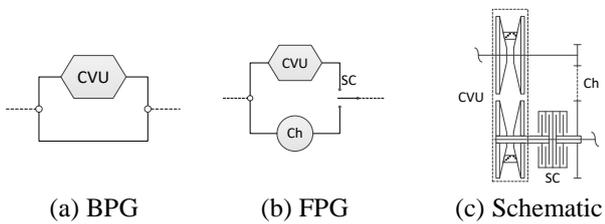
Fig. 4. Viable example of the bypass loop structure
