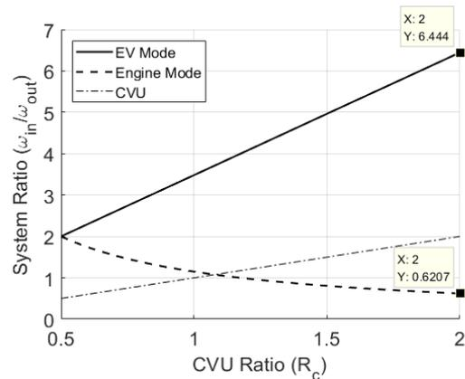
Fig. 13. System ratio in both modes compared with the CVU
