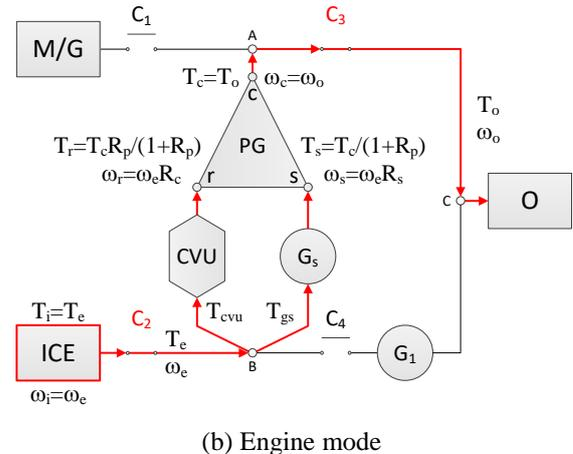
Fig. 11. Torque, speed, and power flow pattern in the two basic operation modes
