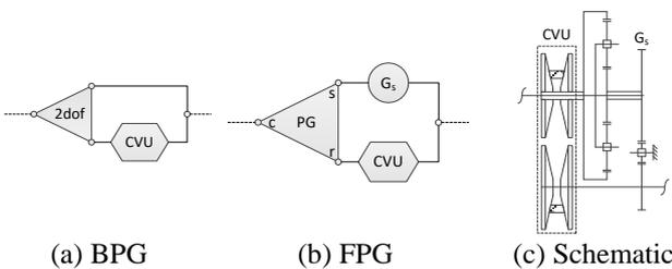
Fig. 5. Viable example of the power-split loop structure
