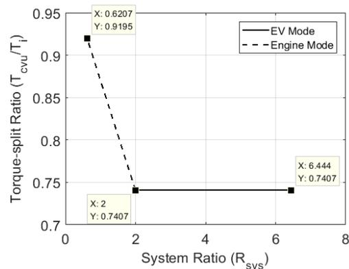
Fig. 14. Variation in the torque-split ratio
