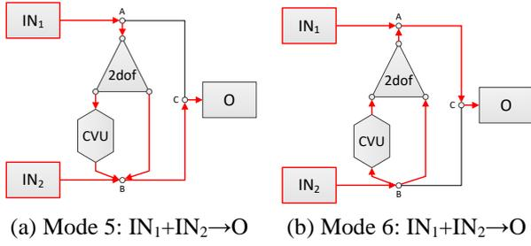
Fig. 9. Power flow patterns with double power sources
