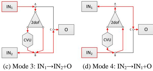
Fig. 8. Power flow patterns with a single power source
