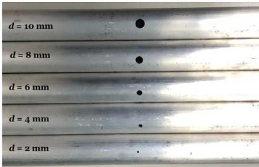
Fig. 3. A picture of round-hole 6061-T6 aluminum alloy tubes with different  $d$ .
