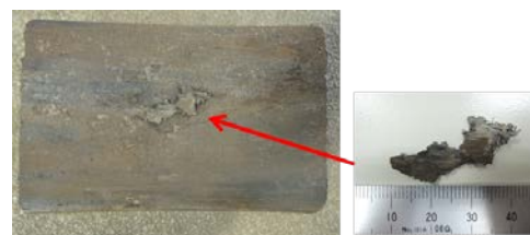
Figure 4: Iron flakes peeled off from the polishers
