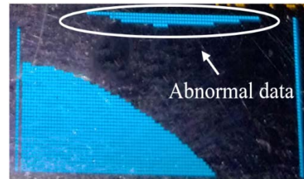
Fig.5. The scene misjudgment of the traditional edge extraction algorithm
