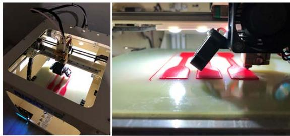
Fig. 1. Printing of test products using a 3D printer.
