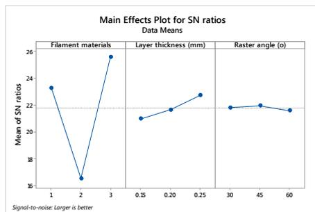
Fig. 5. S / N rates for izod impact.
