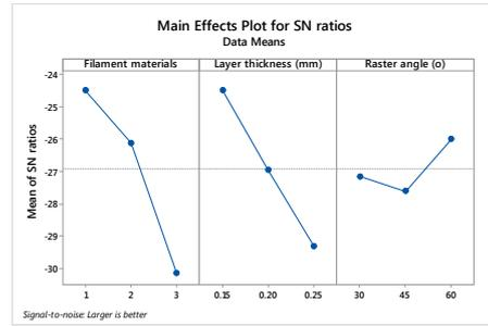
Fig. 4. S / N rates for elongation at break.
