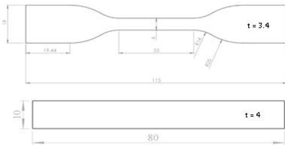
Fig. 2. Dimensions of the tensile and impact strength test samples (mm).
