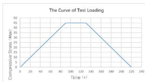
Fig 4-2 High temperature loading curve
