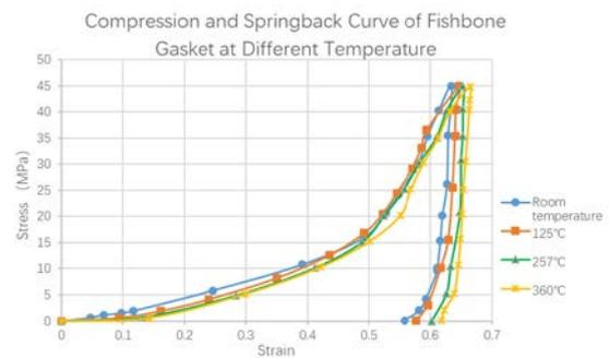
Fig 4-6 Compression springback of fishbone gasket at different temperatures
