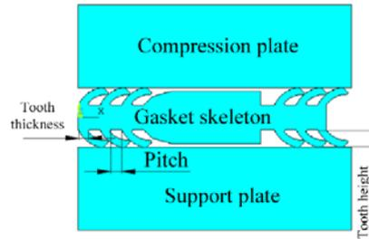
Fig 3-1 ANSYS model of fishbone gasket
