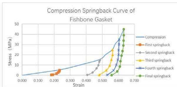
Fig 4-5 The curve of compression springback at room temperature
