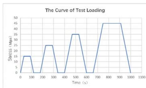
Fig 4-1 Room temperature loading curve
