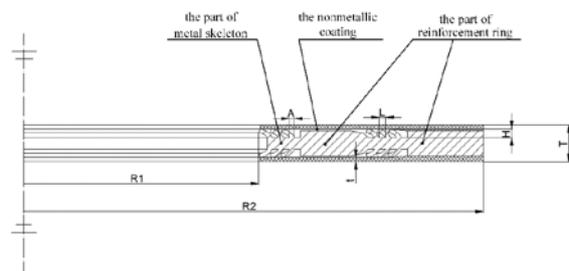
Figure 2-1 Basic structure brief diagram of fishbone gasket
