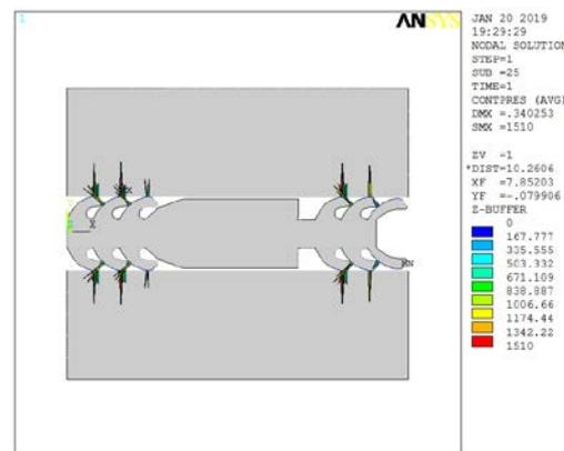
Fig 3-3 Contact stress of fishbone gasket skeleton under compression
