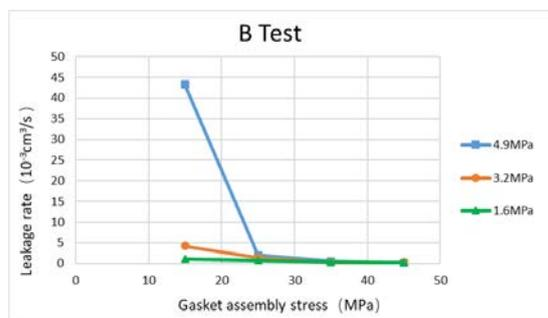
Fig 5-2 The curve of B test leakage rate
