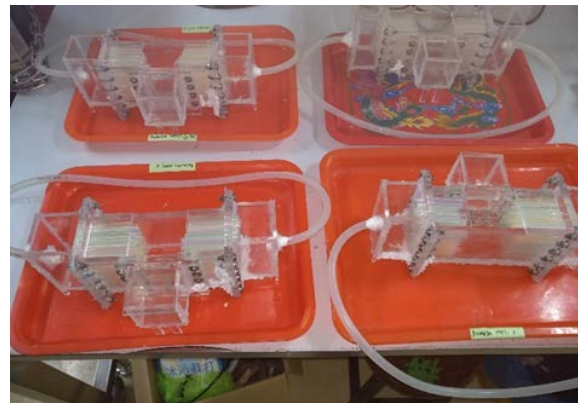
Fig. 1. The honeycomb microbial fuel cells experimental tank.
