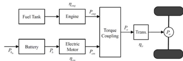
Fig. 2. Parallel PHEV powertrain architecture.
