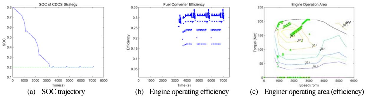
Fig. 7. Simulation results using EV-CS strategy.
