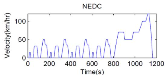
Fig. 4. Driving cycle New European Driving Cycle (NEDC).
