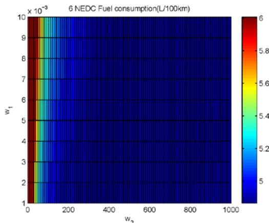
Fig. 9. Fuel consumption with respect to weights  $w_1$  and  $w_2$  from Neural Network for the distribution of fuel consumption.
