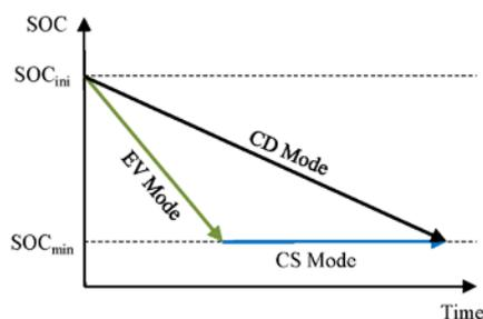
Fig. 1. Driving modes of PHEVs (Wirasingha and Emadi, 2011).
