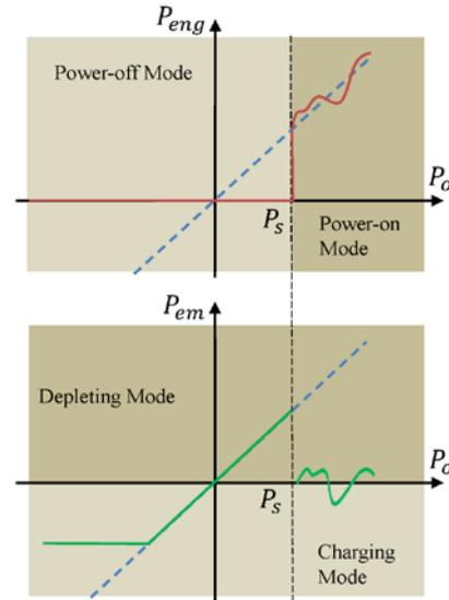
Fig. 3. Engine on/off status for the proposed rule-based power management, where  $P_o = P_{eng} + P_{em}$ .
