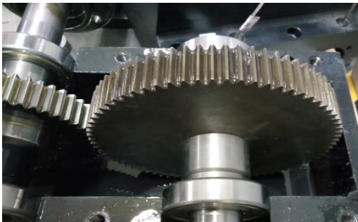
(c) Tooth profile error fault
