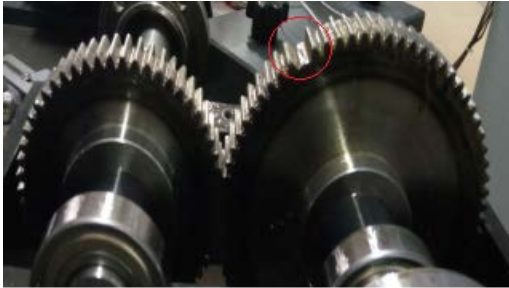
(b) Broken tooth fault
