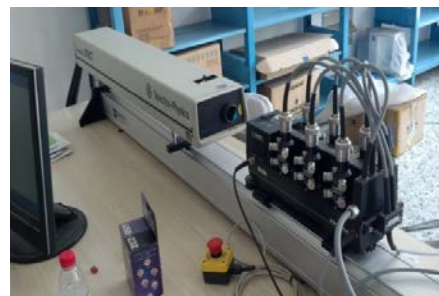
Fig. 2. Laser generator part of the PDA system
