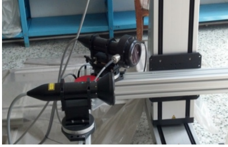
Fig. 3. Laser probe of the PDA system
