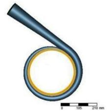
Fig.26. New snail shell 3D drawing
