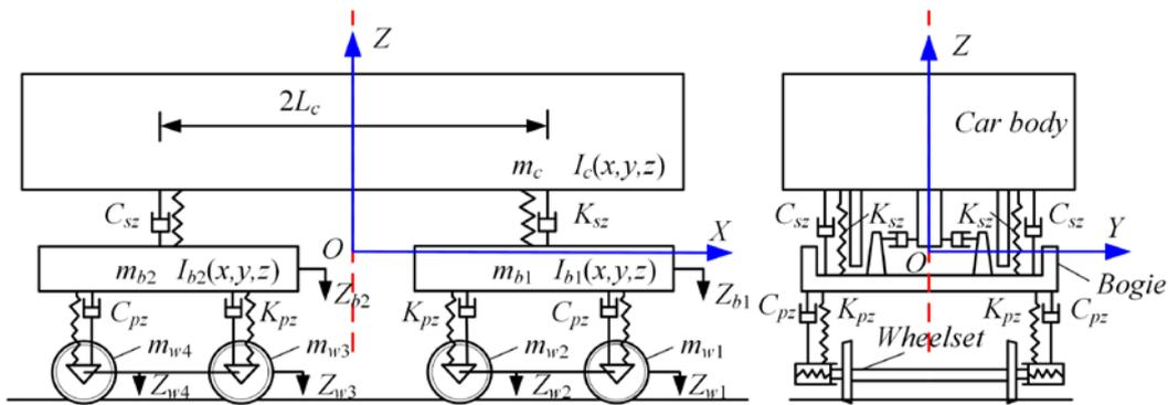
Fig. 1 Vertical dynamics model of a rail vehicle
