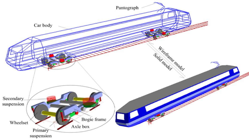
Fig. 4 The multi-body dynamics simulation model of rail vehicle
