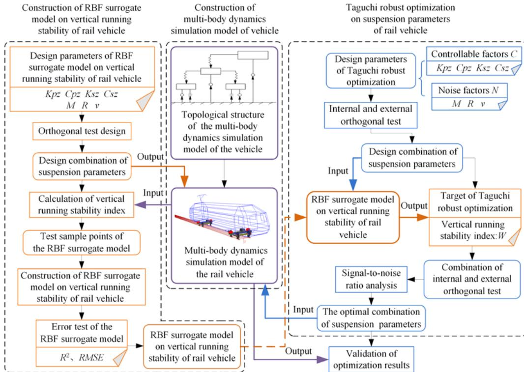
Fig. 2 The procedure of Taguchi robust optimization on suspension parameters
