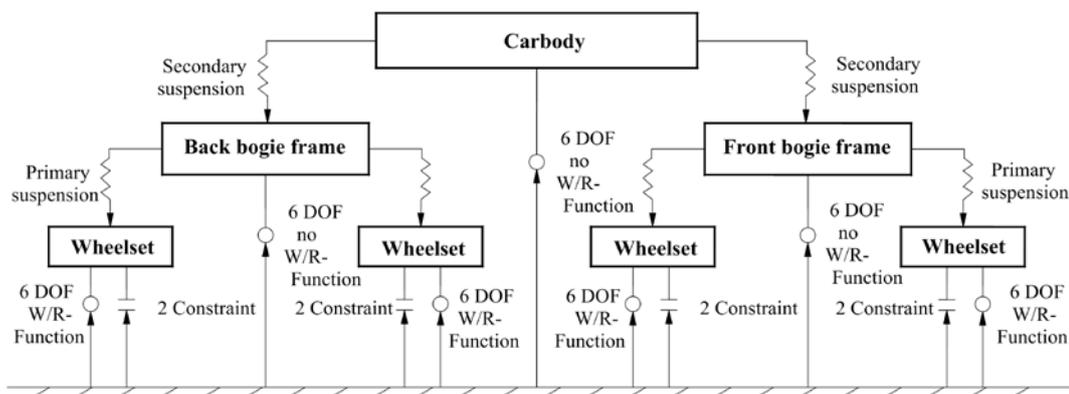
Fig. 3 The topological structure of the multi-body dynamics simulation model of rail vehicle
