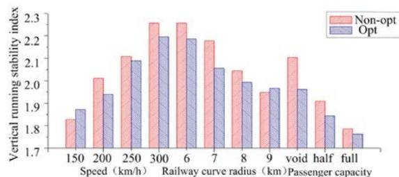
Fig. 9 Comparison of vertical running stability indexes under the influence of noise factors
