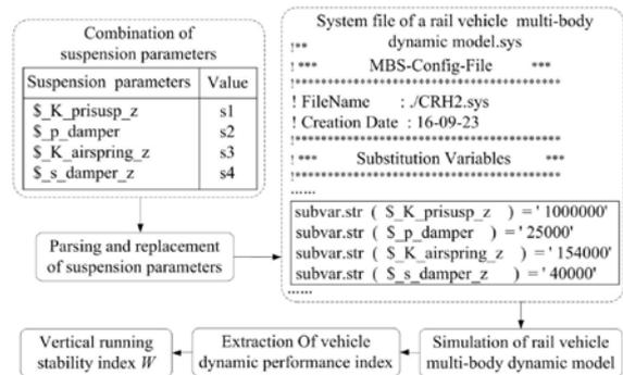
Fig. 5 Simulation process for vehicle running stability
