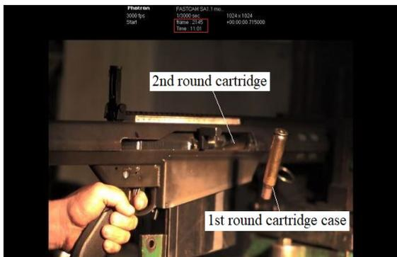
Fig. 19. First round cartridge case ejection and second round cartridge feeding into the barrel chamber from the magazine
