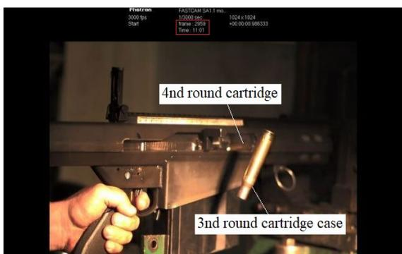
Fig. 21. Third round cartridge case ejection and
