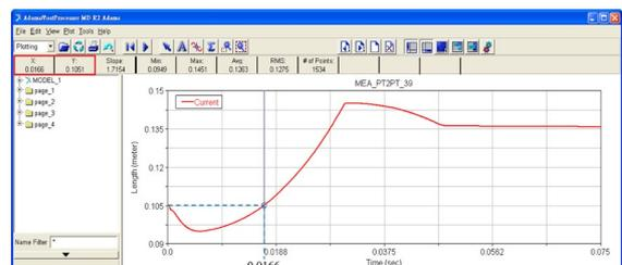
Fig. 14. Bolt starts to unlock from the barrel when  $T = 16.6$  ms
