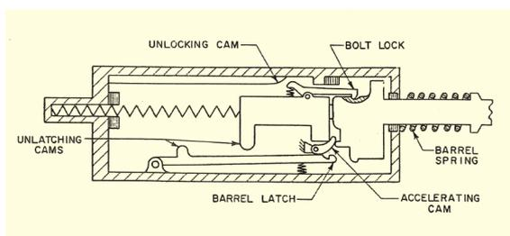
Fig. 2. Schematic representation of a barrel recoil-
