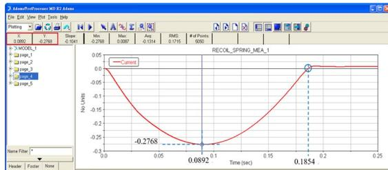
Fig. 15. Bolt carrier recoils backward until the stop position at 89.2 ms and returns forward to the initial position at 185.4 ms
