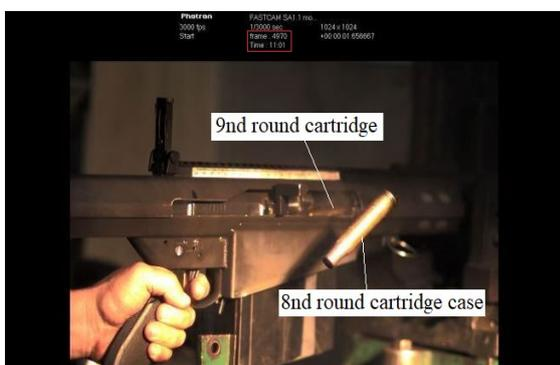
Fig. 26. Eighth round cartridge case ejection and ninth round cartridge feeding into the barrel chamber from the magazine
