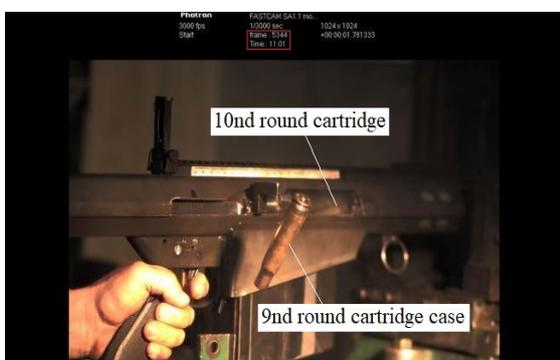
Fig. 27. Ninth round cartridge case ejection and tenth round cartridge feeding into the barrel chamber from the magazine
