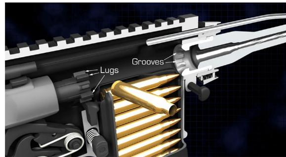
Fig. 3. Schematic representation of the rotary locking device (45Snipers, 2017)
