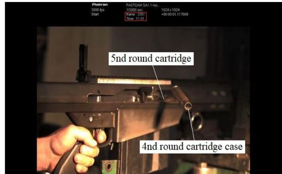
Fig. 22. Fourth round cartridge case ejection and fifth round cartridge feeding into the barrel chamber from the magazine
