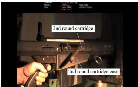
Fig. 20. Second round cartridge case ejection and third round cartridge feeding into the barrel chamber from the magazine
