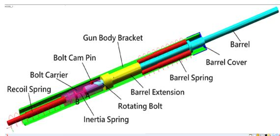
Fig. 5. Concept design graphic of the new firearm mechanism developed in this research
