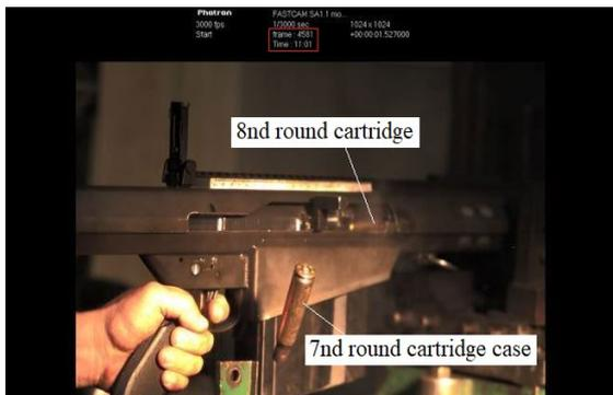
Fig. 25. Seventh round cartridge case ejection and eighth round cartridge feeding into the barrel chamber from the magazine
