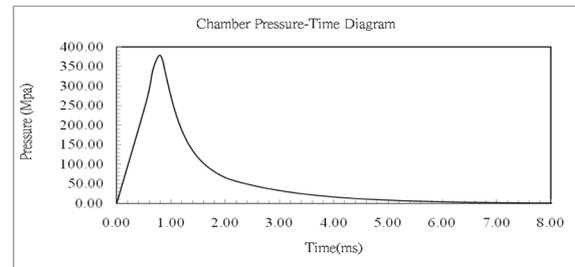
Fig. 4. Relationship of barrel mean chamber pressure versus time
