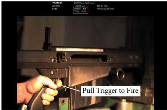
Fig. 18. Shooter pulled the trigger to start nine rounds of fully automatic shooting
