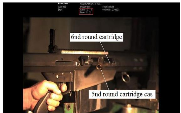
Fig. 23. Fifth round cartridge case ejection and sixth round cartridge feeding into the barrel chamber from the magazine
