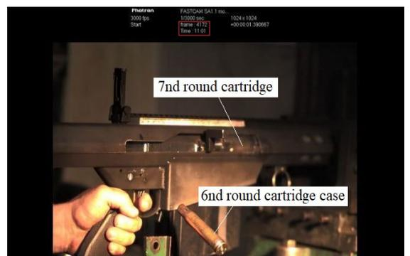
Fig. 24. Sixth round cartridge case ejection and seventh round cartridge feeding into the barrel chamber from the magazine
