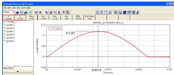
Fig. 16. Maximum recoil distance of the barrel is 11.8 cm when  $T = 31.4$  ms
