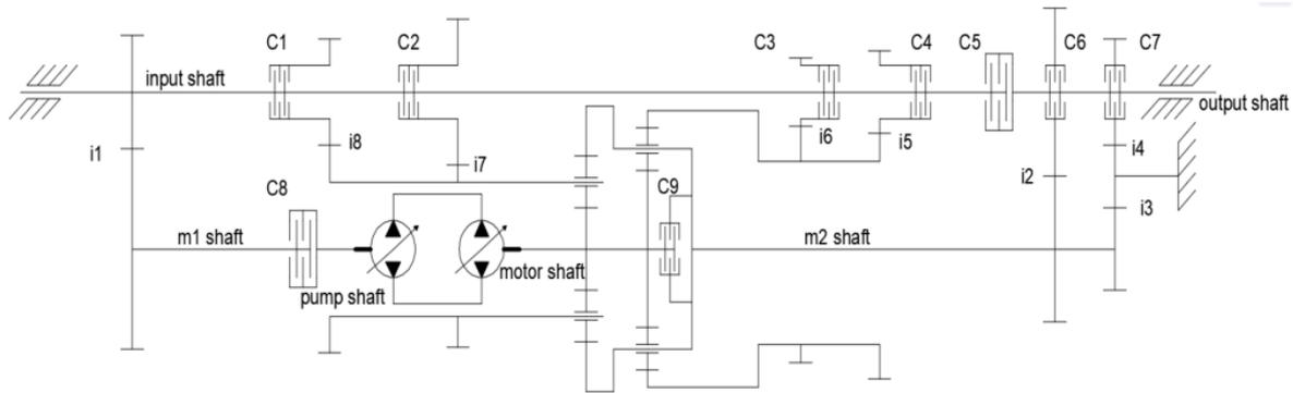
Fig. 1. HMCVT schematic diagram.
