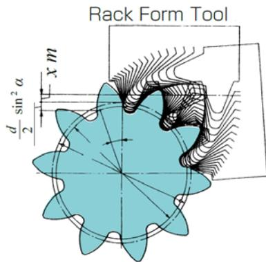
Figure 6. Generation of positive shifted gear ( $\alpha=20^\circ$ ,  $z=10$ ,  $x=+0.5$ )
