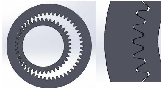
Figure 4. Engagement of the gear set with 9 teeth difference ( $m=1, z_1=41, z_2=50$ )
