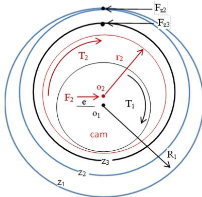
Figure 9. The loading analysis of the gear sets.
