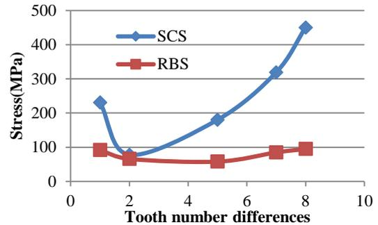
Figure 13. Varying of the stresses corresponding to the tooth number differences
