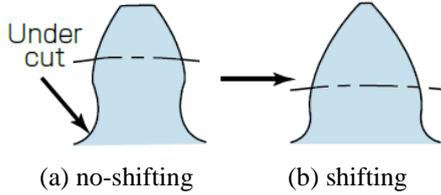
Figure 5. Comparison of the tooth's profiles
