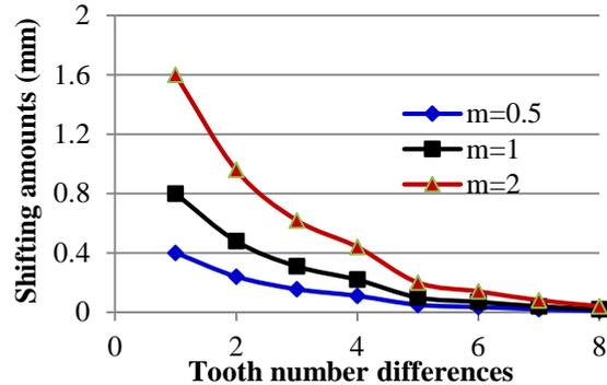
Figure 8. The proper shifting amounts for the gear sets with various tooth differences
