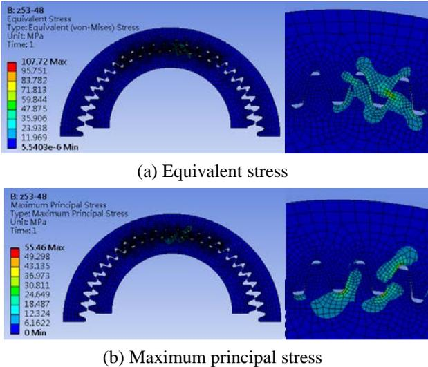
Figure 12. Stresses of the front gear set z(48-53)
