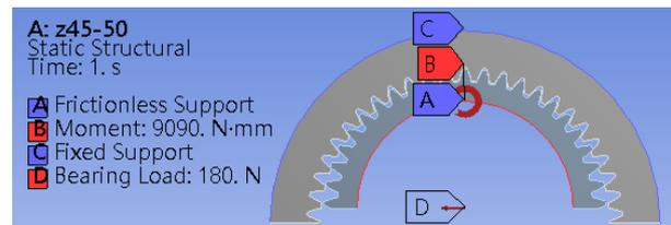
Figure 10. Settings of the supports and the loadings
