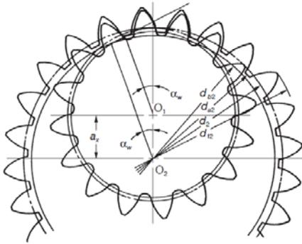
Figure 3. Engaging of the inner and the external gears
