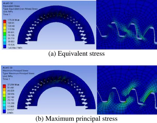
Figure 11. Stresses of the rear gear set z(45-50)
