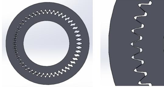
Figure 7. Engagements of the profile shifted gears ( $m=1$ ,  $z_1=49$ ,  $z_2=50$ ,  $x_1=0$ ,  $x_2=0.8$ )
