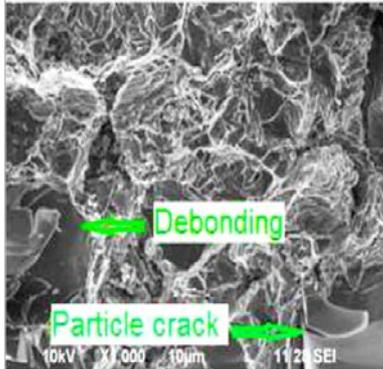
Fig. 11. SEM of the fractured Al/7.5 wt.% CSA/2.5 wt.% SiC<sub>p</sub> composites after tensile test
