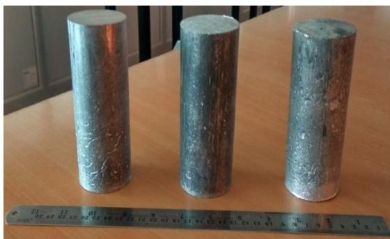
Fig. 2. Squeeze casting samples
