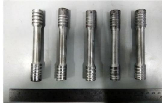
Fig. 3. Tensile test specimens
