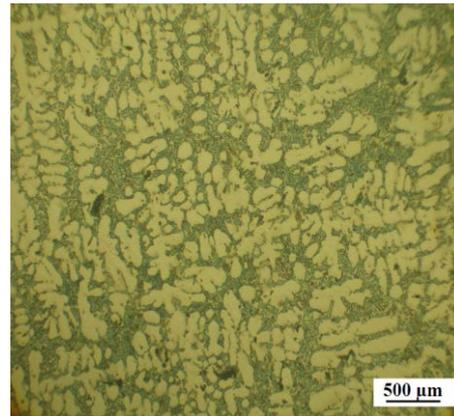
Fig. 8. Microstructure for HAMCs at 2.5 wt.% CSA + 7.5 wt.% SiC<sub>p</sub> (squeeze pressure of 50 MPa, pouring temperature of a 700°C and mould temperature of 250°C are fixed)
