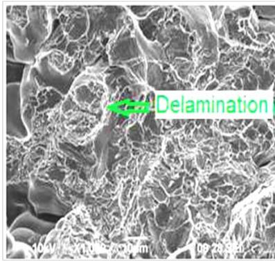
Fig. 9. SEM of the fractured Al/2.5 wt.% CSA/7.5 wt.% SiC<sub>p</sub> composites after tensile test
