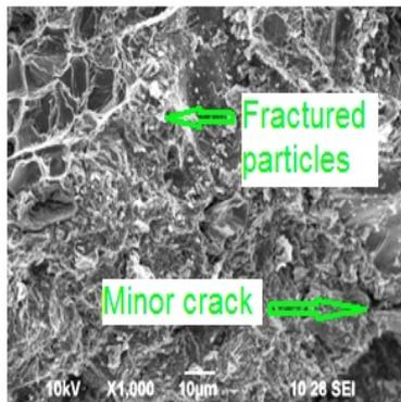
Fig. 10. SEM of the fractured Al/5 wt.% CSA/5 wt.% SiC<sub>p</sub> composites after tensile test
