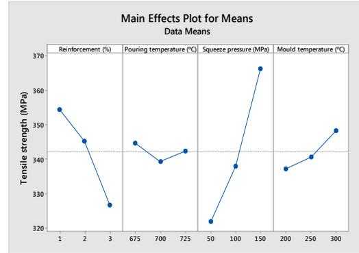
Fig. 4. Main Effect plot of the response - Tensile strength
