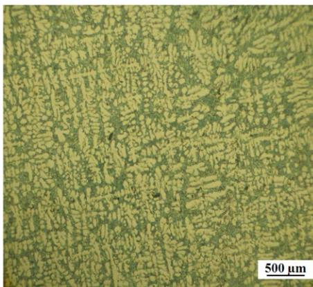
Fig. 7. Microstructure for HAMCs at 2.5 wt.% CSA + 7.5 wt.% SiC<sub>p</sub> (squeeze pressure of 100 MPa, pouring temperature of a 700°C and mould temperature of 250°C are fixed)
