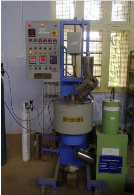
Fig. 1. Squeeze casting experimental set-up
