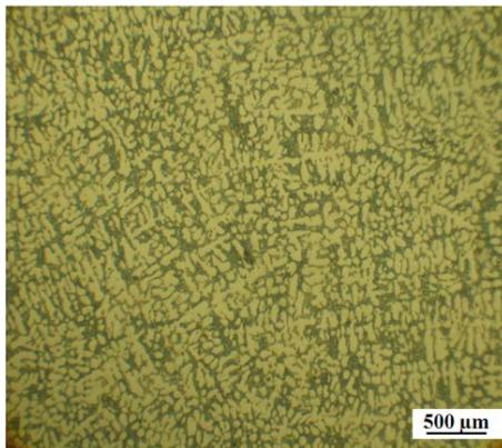
Fig. 6. Microstructure for HAMCs at 2.5 wt.% CSA + 7.5 wt.% SiC<sub>p</sub> (squeeze pressure of 150 MPa, pouring temperature of 700°C and mould temperature of 250°C are fixed)
