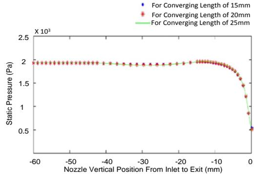
Fig. 10. Static Pressure Profile for Different Converging Length's
