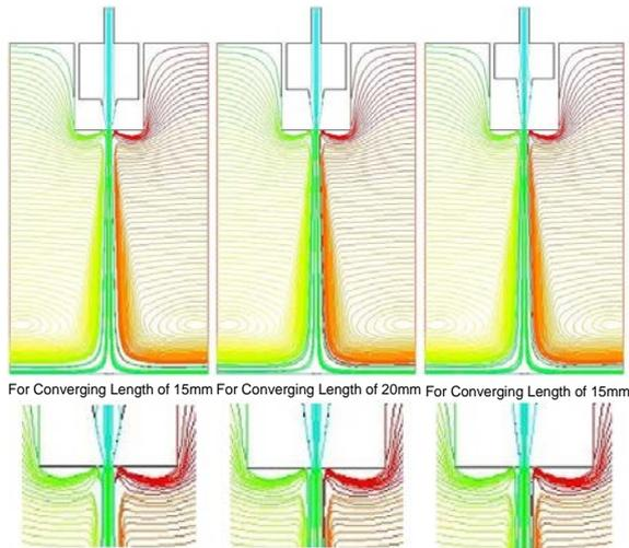
Fig. 12. Flow Pattern for Different Converging Lengths
