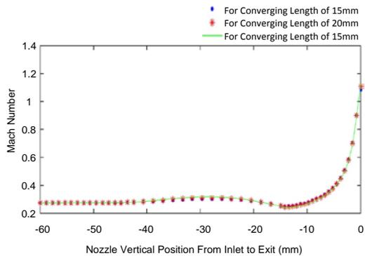
Fig. 11. Mach Number Profile for Different Converging Length's
