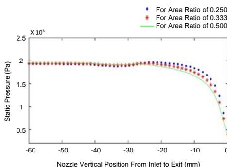
Fig. 4. Variation of Static Pressure of Different Area Ratio's
