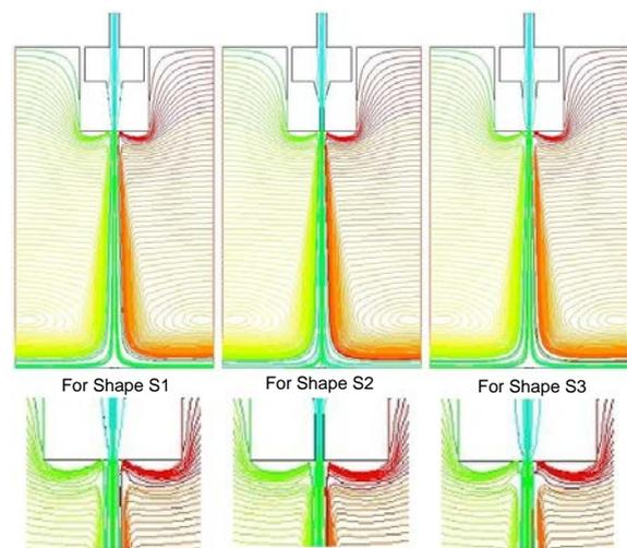
Fig. 16. Flow Pattern for Different Nozzle Shapes
