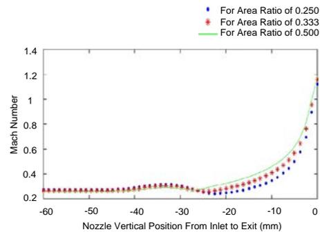
Fig. 5. Variation of Mach Number for Different Area Ratio's
