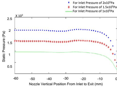
Fig. 7. Static Pressure Profile for Different Inlet Pressures.
