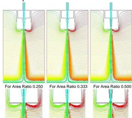
Fig. 6. Flow Pattern for Different Area Ratios
