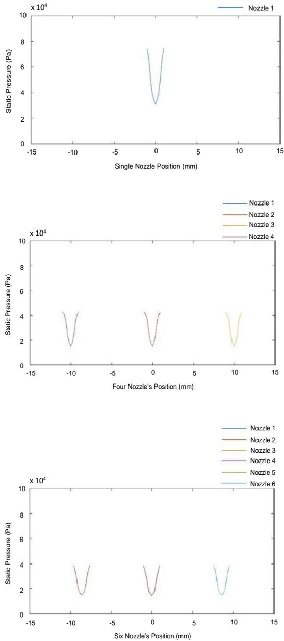
Fig. 17. Static Pressure for Different Nozzle Blocks.
