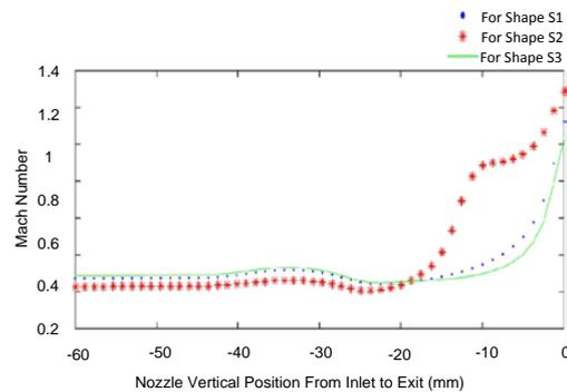
Fig. 15. Mach Number Profile with Different Nozzle Shapes
