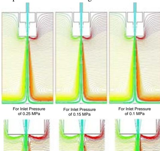
Fig. 9. Flow Pattern for Different Inlet Pressures
