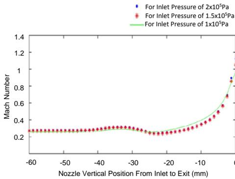
Fig. 8. Mach Number Profile for Different Inlet Pressures
