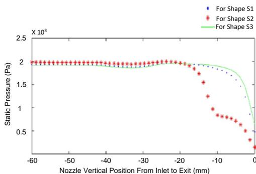
Fig. 14. Static Pressure Profile for Different Nozzle Shapes
