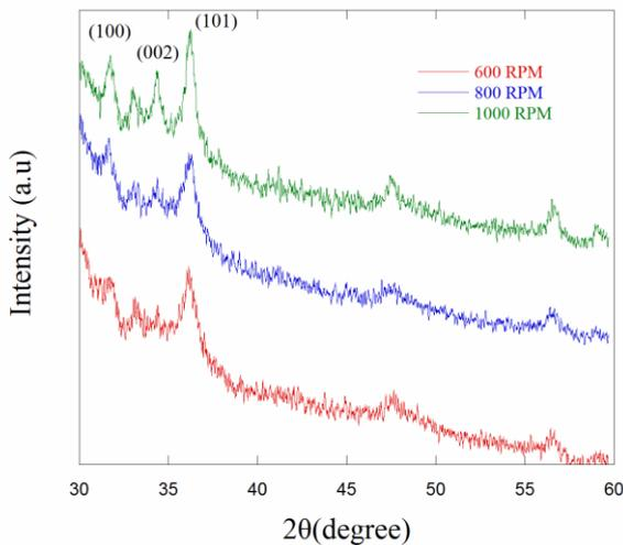
Fig. 4 The XRD of AlN doped ZnO thin film deposited on the copper substrate with different speeds of spin-coating (600, 800, 1000 rpm)
