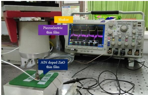
Fig. 7 The apparatus of the force feedback testing system
