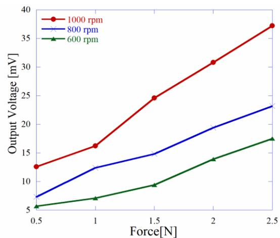
Fig. 8 Voltage response of AlN doped ZnO thin film tactile sensor on the PI substrate
