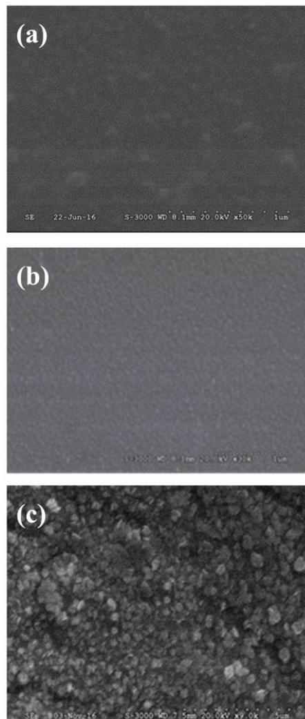
Fig. 6 The SEM photograph of AlN doped ZnO thin film, speed of spin-coating (a) 600 rpm (b) 800 rpm (c) 1000 rpm
