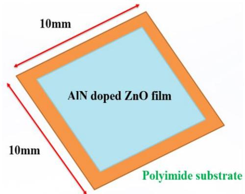
Fig. 2 The schematic diagram of tactile sensor based on AlN doped ZnO thin films
