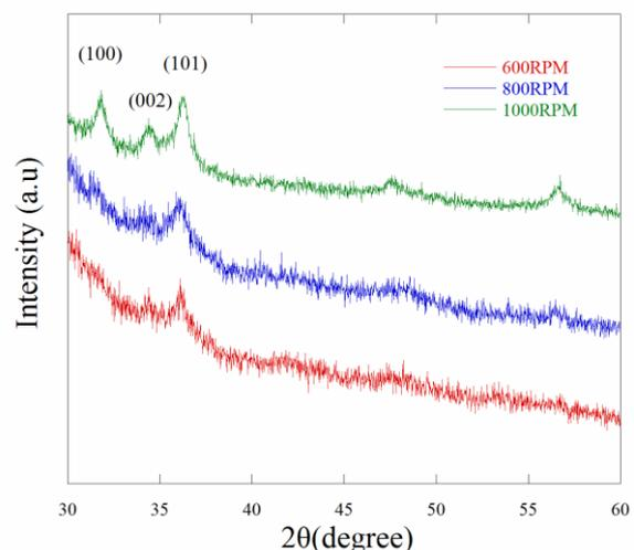
Fig. 3 The XRD of AlN doped ZnO thin films deposited on the PI substrate with different speeds of spin-coating (600, 800, 1000 rpm)
