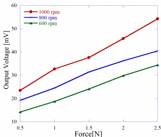
Fig. 9 Voltage response of AlN doped ZnO thin film tactile sensor on the copper substrate
