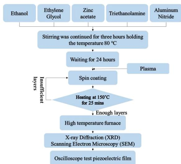
Fig. 1 The flow chart for the preparation of AlN doped ZnO thin films
