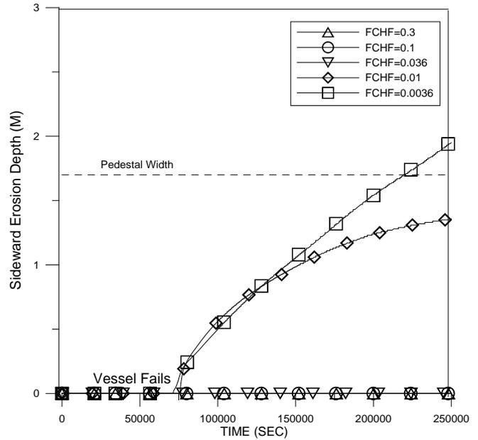
Fig. 8 Sideward Erosion Depth for Different FCHF in the SBRC-PF-R-N Sequence
