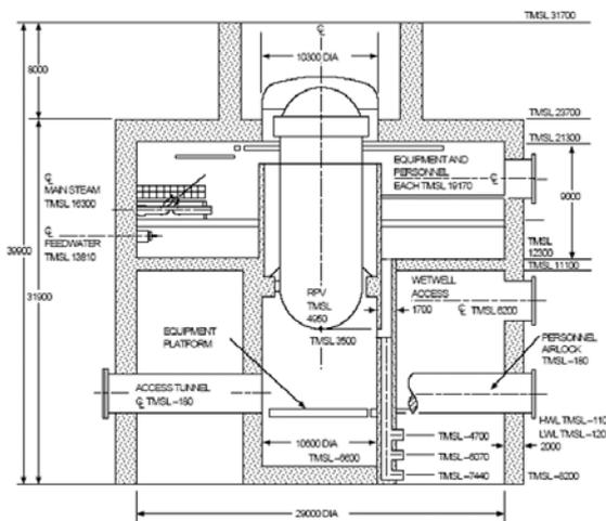
Fig. 1 Lungmen Containment Configuration
