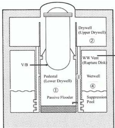
Fig. 3 MAAP5 Containment Nodalizations
