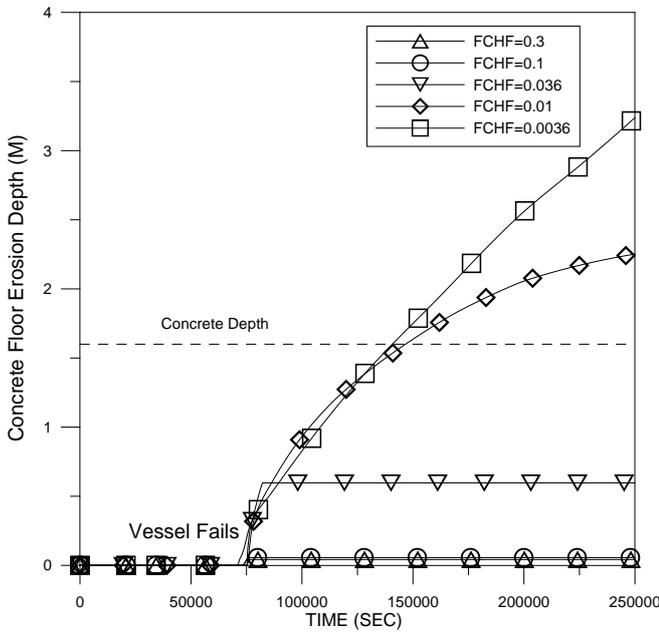
Fig. 7 Downward Erosion Depth for Different FCHF in the SBRC-PF-R-N Sequence
