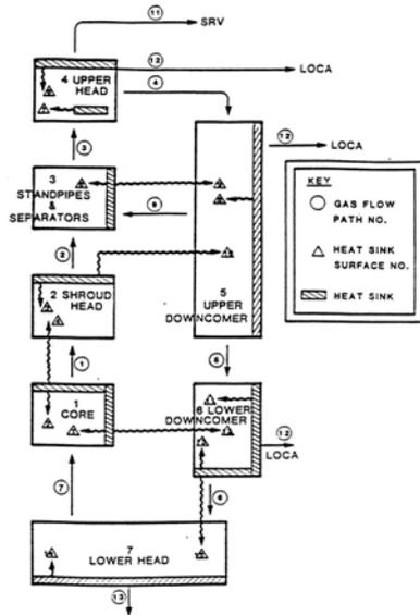
Fig. 2 MAAP5 Reactor Nodalizations
