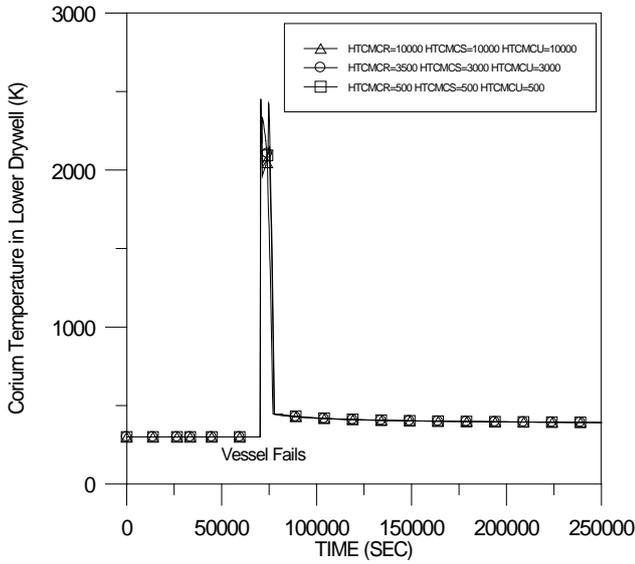
Fig. 6 Average Temperature of Corium in Lower Drywell for Different Heat Transfer Coefficients in the SBRC-PF-R-N Sequence
