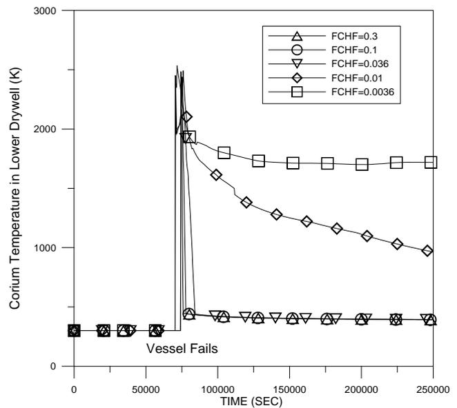
Fig. 9 Average Temperature of Corium in Lower Drywell for Different FCHF in the SBRC-PF-R-N Sequence
