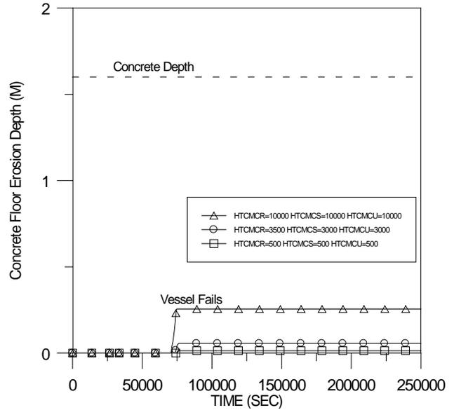
Fig. 4 Downward Erosion Depth for Different Heat Transfer Coefficients in the SBRC-PF-R-N Sequence
