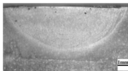
Fig. 2 Near surface porosity of weld zone
