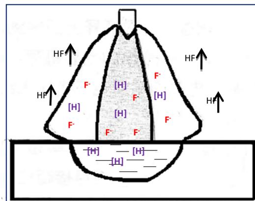
Fig.5 Hydrogen fluoride reaction diagram
