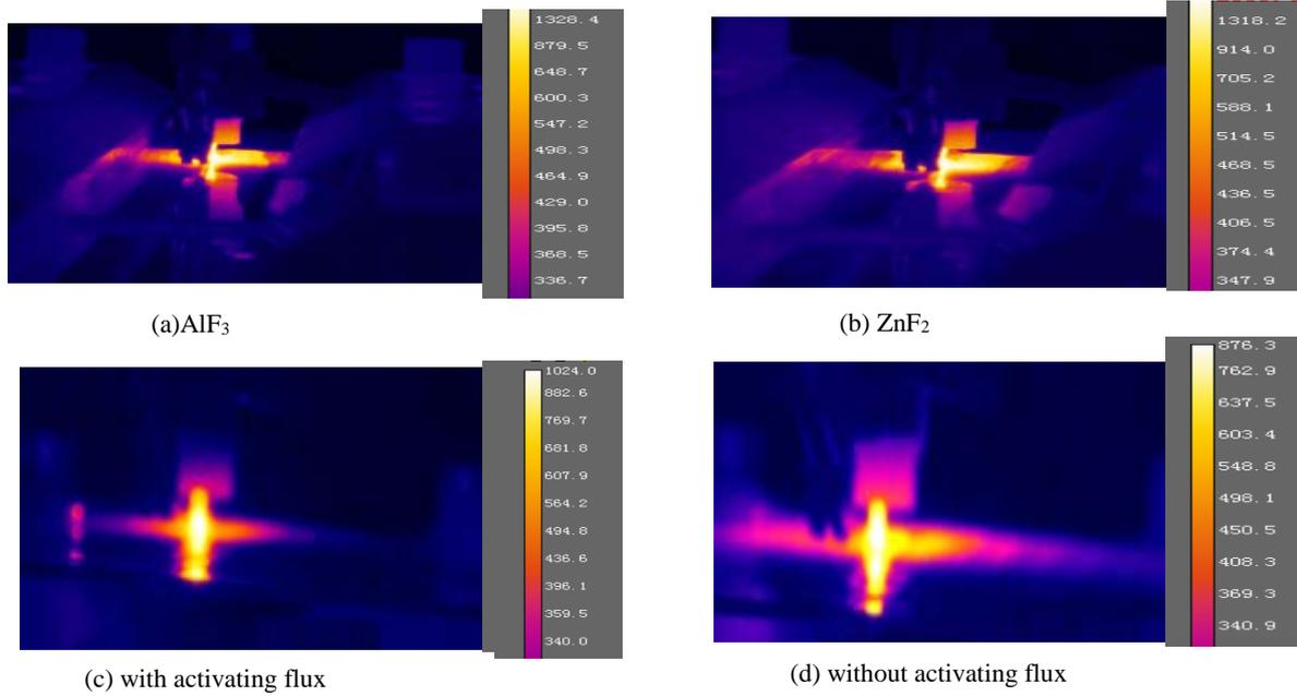
Fig.6 Infrared thermography of the temperature field of welded joints
