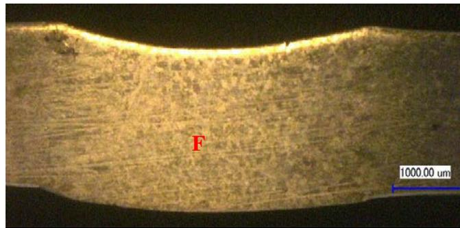
Fig. 9 Weld forming of DCSP A-TIG welding
