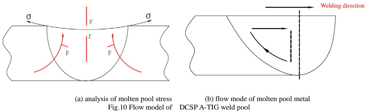
as shown in Fig. 10(b), which was beneficial to inhibit the generation of air holes. At the same time, the increase of heat input increased the radial component of arc, made the liquid metal in molten pool flow from center to both sides, made a part of melting heat transfer to the periphery of molten pool continuously, increased the size of molten pool, and helped bubble float out.
