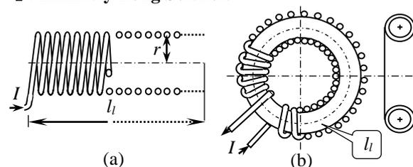
Fig. 1 (a) Infinitely long solenoid. (b) Toroidal winding. [10]
