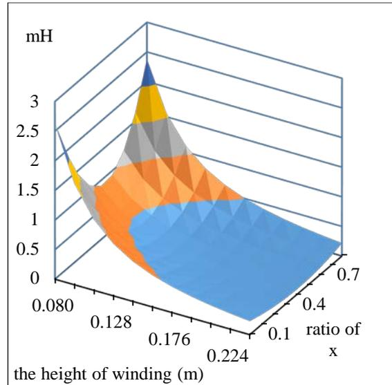
Fig. 4 Trend of the magnitudes of the leakage inductance with the height of winding and the distributive ratio of secondary winding
