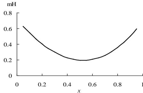
Fig. 3 The calculated values of leakage inductance vary with the value of  $x$ .
