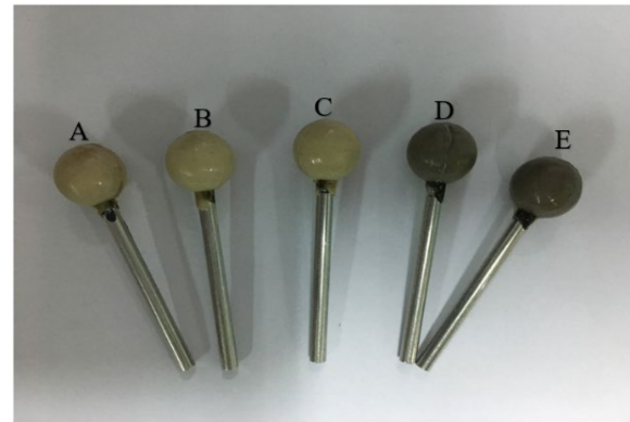
Fig. 9. Photo of the fabricated lab-made polishing balls.
