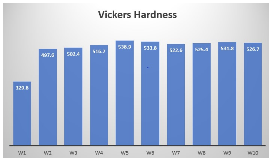
Fig. 2. Changes of average hardness by heat treatment in samples.
