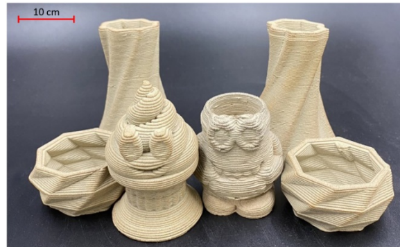
Fig. 5. Printed parts of the recycle oyster shell and clay
