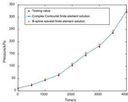
Fig.3. Changing curves of internal pressure
