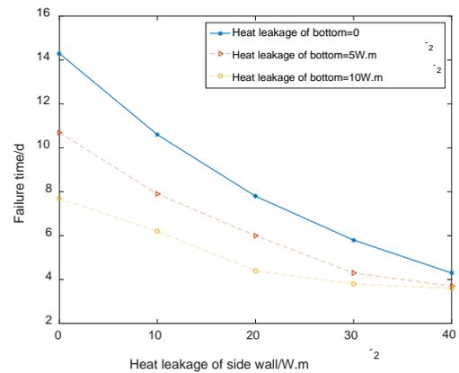
Fig.4. Failure time changing curve of LNG tank with heat leakage
