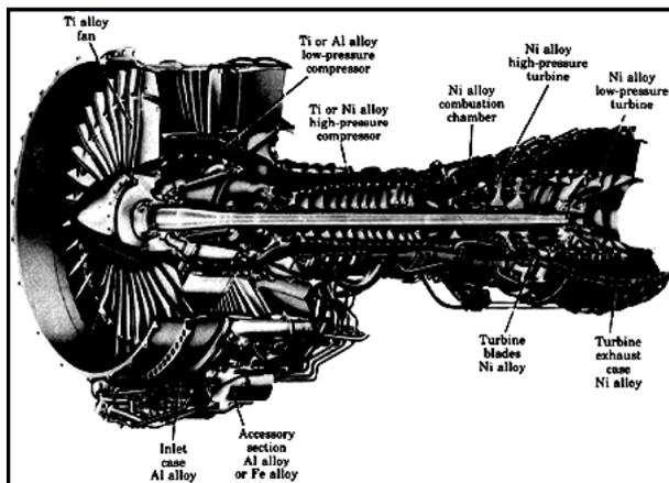
Figure 1. Typical Material Distribution in Jet Engine Flake (2006)
