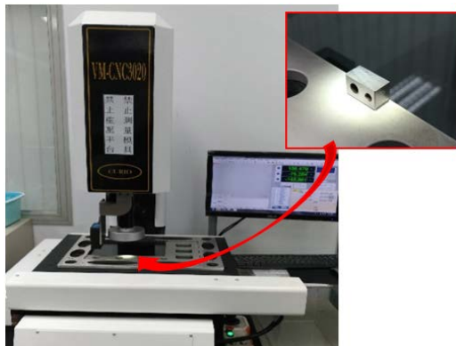
Fig 16 The processed gate inserts are measured with 2.5D image measuring instrument. The gates with \theta=0 and \theta=45 have lengths of 0.69 mm and 1.18 mm along Y-axis, respectively.
