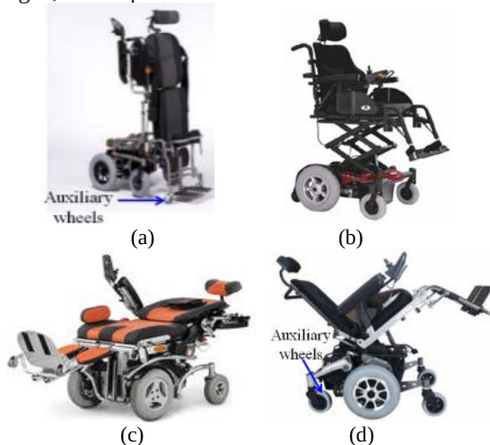
Fig. 1. Single functional wheelchairs: (a) Standing wheelchair; (b) Lifting wheelchair; (c) Lying wheelchair; (d) Tilting wheelchair
