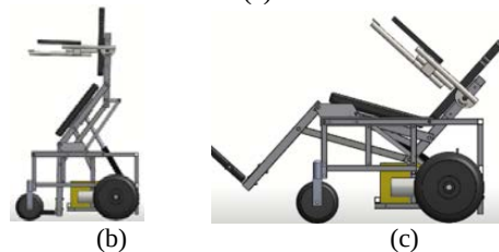
Fig. 19. Side views of the wheelchair with standing and tilting functions: (a) Sitting posture; (b) Standing posture; (c) Tilting posture
