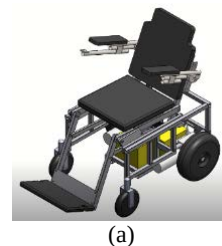
Fig. 19. Side views of the wheelchair with standing and tilting functions: (a) Sitting posture; (b) Standing posture; (c) Tilting posture
