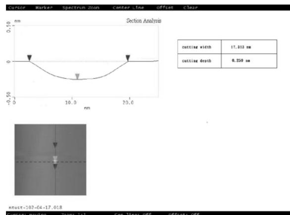
**Fig. 2.** Partial AFM experimental results under the following conditions: a cutting depth interval of approximately 0.05 nm, sapphire substrate dipped in 50% slurry for 90 min at 23°C, down force of 9.55  $\mu\text{N}$ , cutting depth of 0.250 nm, and cutting width of 17.313 nm
