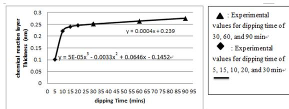
**Fig. 4.** Regression equation and curve for various dipping durations and chemical reaction layer thicknesses (slurry volume concentration: 50%; temperature: 23 °C)
