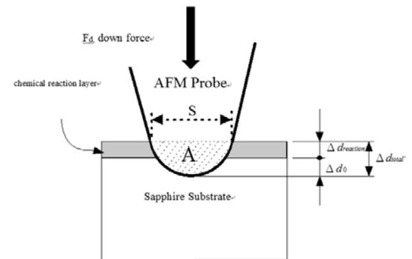
**Fig. 1.** Schematic diagram of chemical reaction layer
