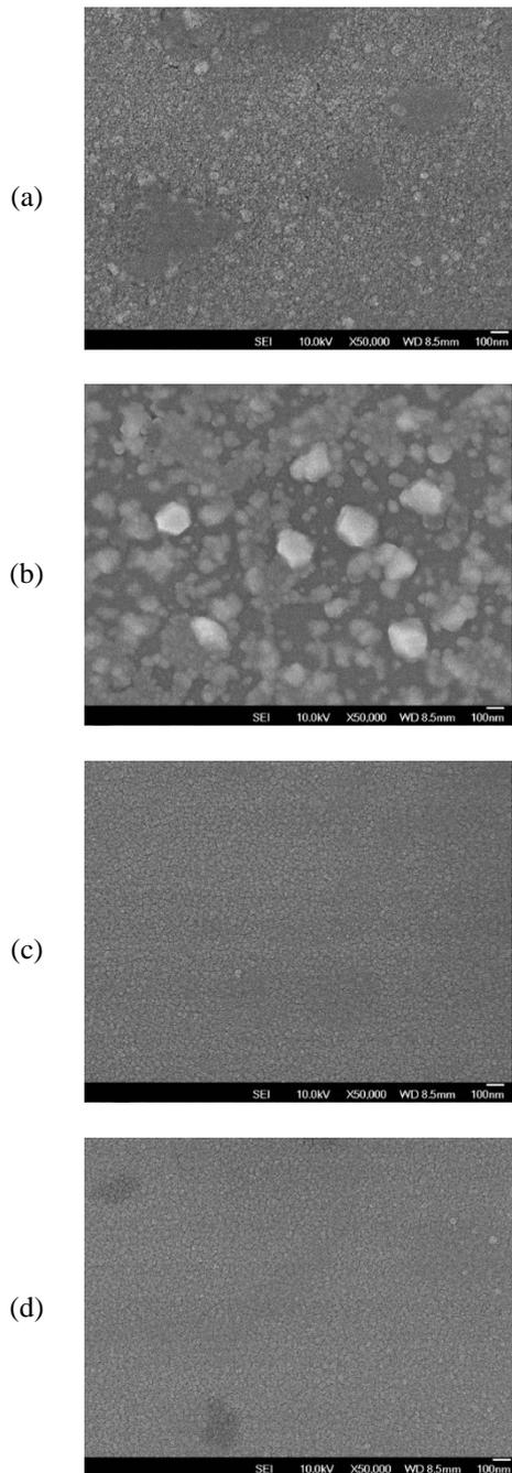
Figure 3. Scanning electron micrograph of (a) Ag/AZO/SnOx/glass before heat treatment, (b) Ag/AZO/SnOx/glass after heat treatment, (c) SnOx/NiCrOx/Ag/AZO/SnOx/glass before heat treatment and (d) SnOx/NiCrOx/Ag/AZO/SnOx/glass after heat treatment.
