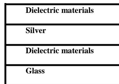
Figure 1. Basic silver-based sandwich structure of low-emissivity glass.
