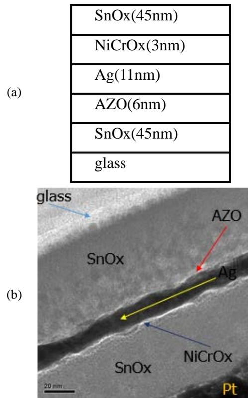
Figure 2. (a) Schematic and (b) produced diagram on cross section of  $\text{SnOx}/\text{NiCrOx}/\text{Ag}/\text{AZO}/\text{SnOx}/\text{glass}$ .
