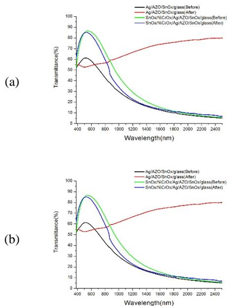
Figure 5. (a) Transmittance and (b) reflectance spectra of Ag/AZO/SnOx/glass and SnOx/NiCrOx/Ag/AZO/SnOx/glass samples before and after heat treatment.
