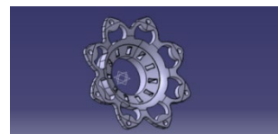
Fig. 5. Improved rear spoke 3D model
