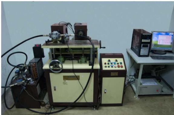
Figure 18 Gear pump test machine
