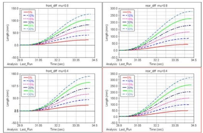
Fig.8 Deviation by unequal braking force of front and rear wheels
