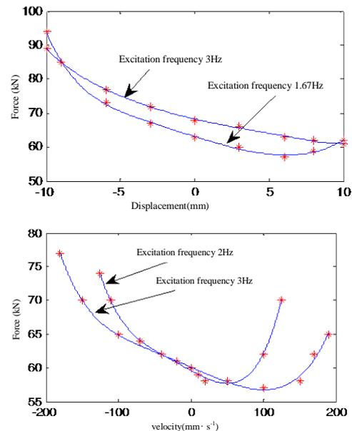
Fig.5 Experimental curve of rear suspension working characteristics
