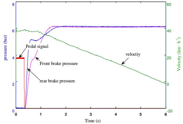
Fig.12 Truck service brake test (4th group)
