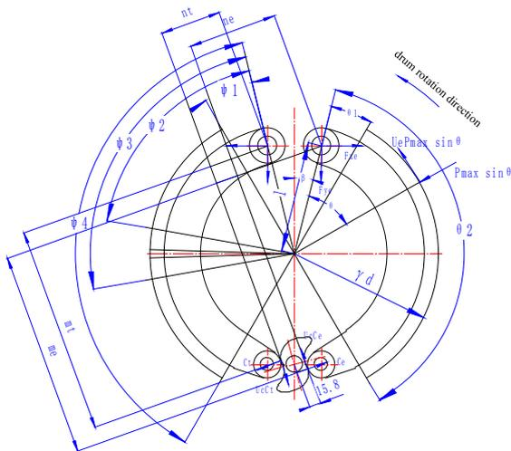
Fig.2 The friction plate force diagram
