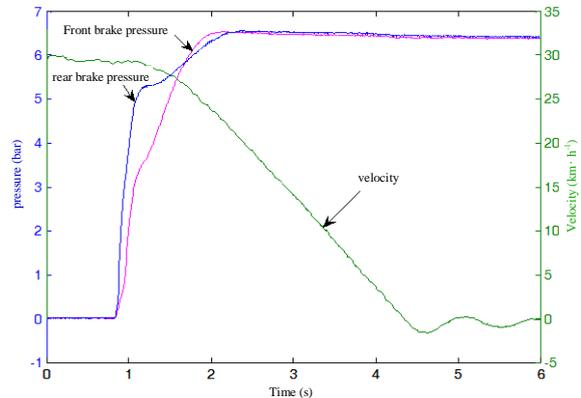
Fig.13 Emergency brake test (2th group)
