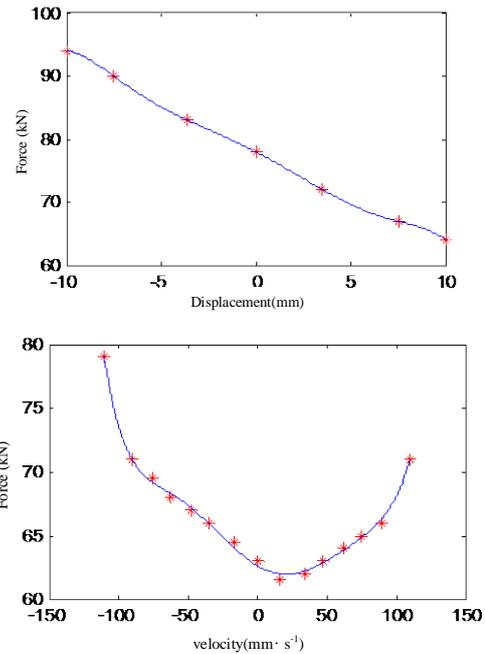
Fig.4 Experimental curve of working characteristics of front suspension (exciting frequency is 1.67 Hz)
