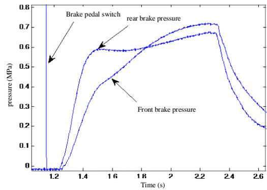
Fig.7 Brake pressure test curve
