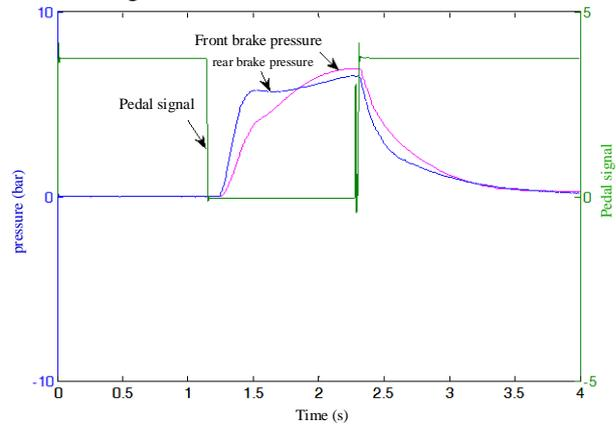
Fig.15 Service brake system pressure response time
