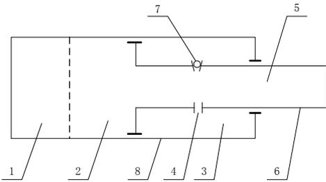
Fig.3 Suspension cylinder installation and structure
